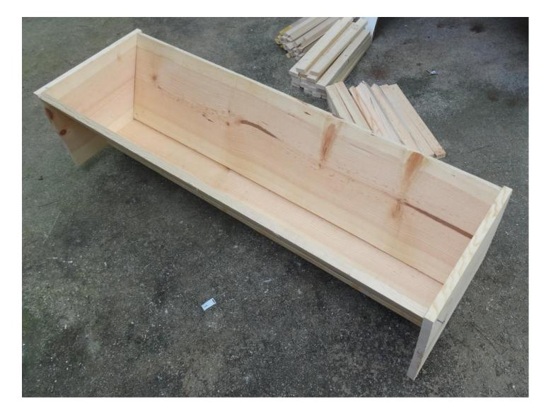
You need to pay some attention to spreading the side boards and make sure that the sides do not project above the end boards. The dimensions given on material list ensure that your ends should look like those above.
