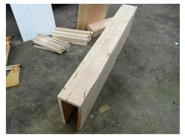
Nail the bottom to the two sides using large finishing nails (don't use screws on bottom). Space the nails at approximately 7" o.c. This will initially look like a U-shaped trough x  $3'-10 \frac{1}{2}$ " long.
